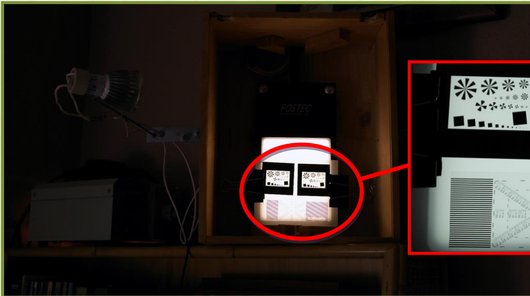
LED front-illuminated target High resolution paper (not good due to light fallout issues)
